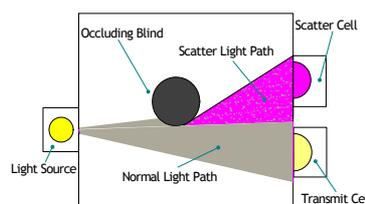
Figure 2 - Schematic of OCM working according to Mie theory. Light only enters the red band because of scattering by solid particles.
