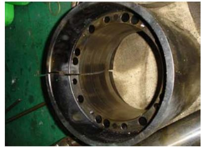
Figure 2 - Severe fracture of piston skirt caused by thermal hoop stress.
