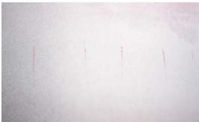
Figure 1 - Pattern of hairline crankshaft cracks revealed by dye penetrant.
